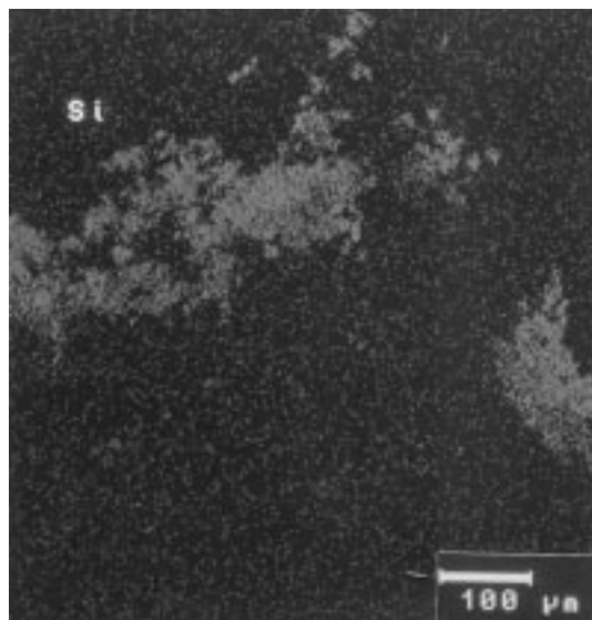
Fig. 8 Secondary electron image of the fractured coating and the nickel-rich layer together with the x-ray mappings for silicon
